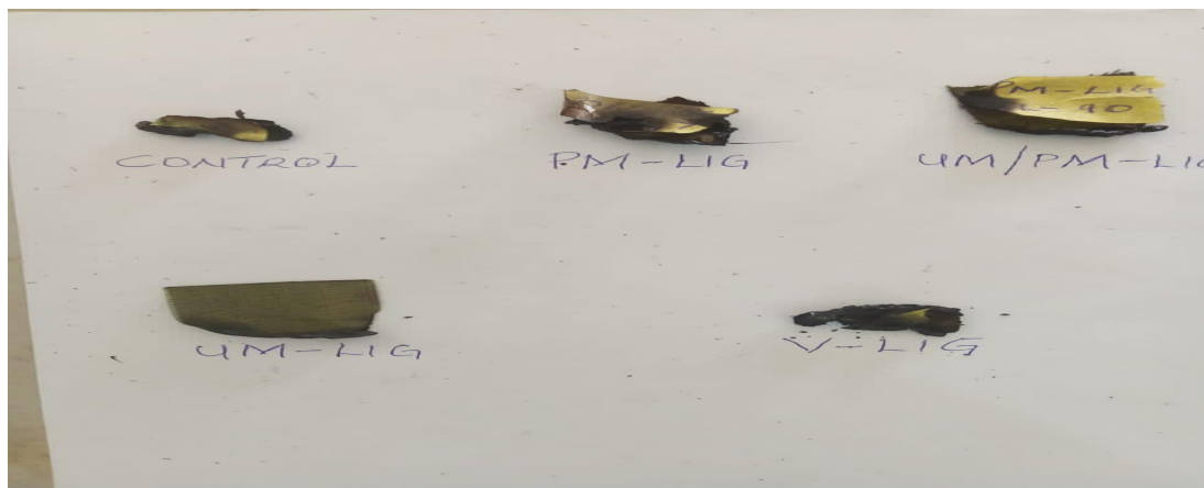
Figure 5.0: Samples after UL-90HB test.
